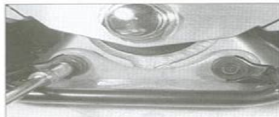
2.10c. Remove the mounting bolts at the front of the tank ...
