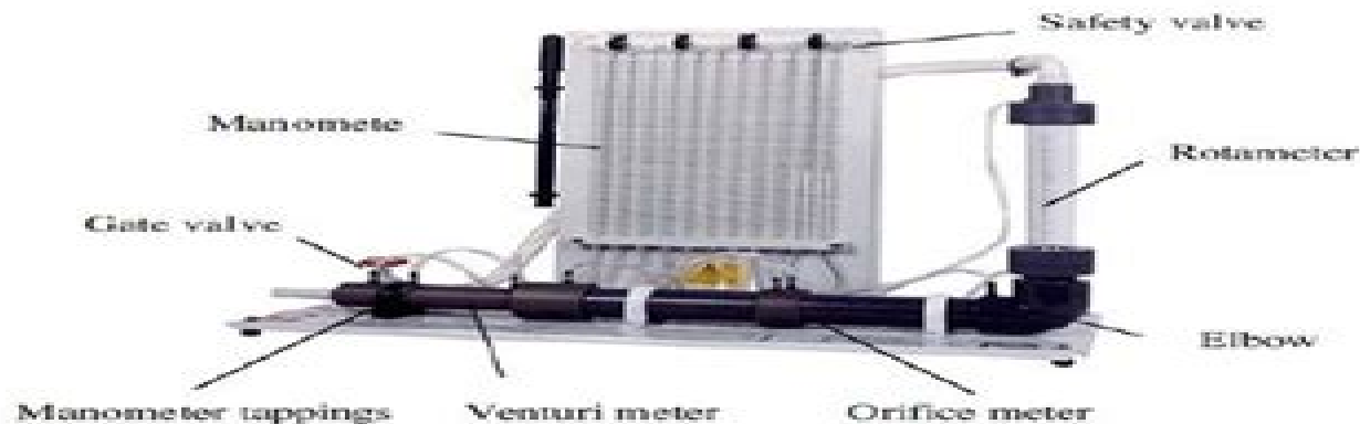
Figure 1. Flow measurement apparatus
