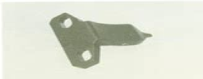
This tool is necessary to replace valve adjusting pads. This can also be used for the XS750.
