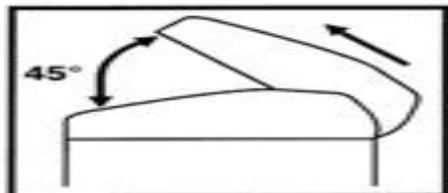
To remove cover, open 45 degrees and slide forward. To replace cover, align attachment hooks into hinge on back of bread maker. Cover should move freely when properly attached.
