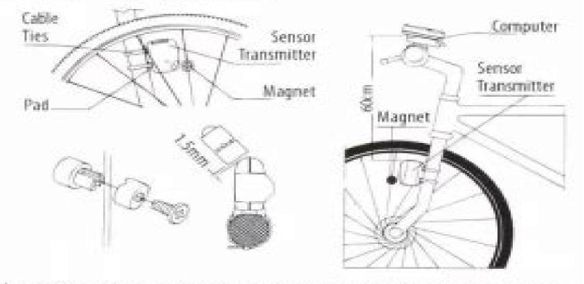
Attach the sensor transmitter to the left fork blade, the distance between com and the sensor can not exceed 60cm, the closer the better. Using the shims to a the diameter, and the cable ties (shown in mounting shoe section) to tie to the
