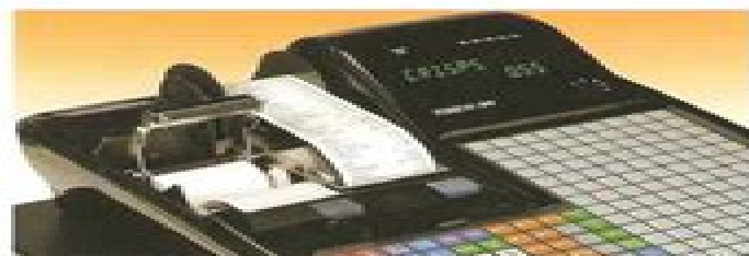
'Drop-in' paper loading mechanism helps users to change paper instantly.
