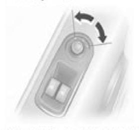
Select the relevant exterior mirror and adjust it by swivelling the control.
