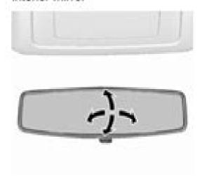
To adjust the mirror, move the mirror housing in the desired direction. Interior mirror, Wide view mirror \$\phi\$ 40.
