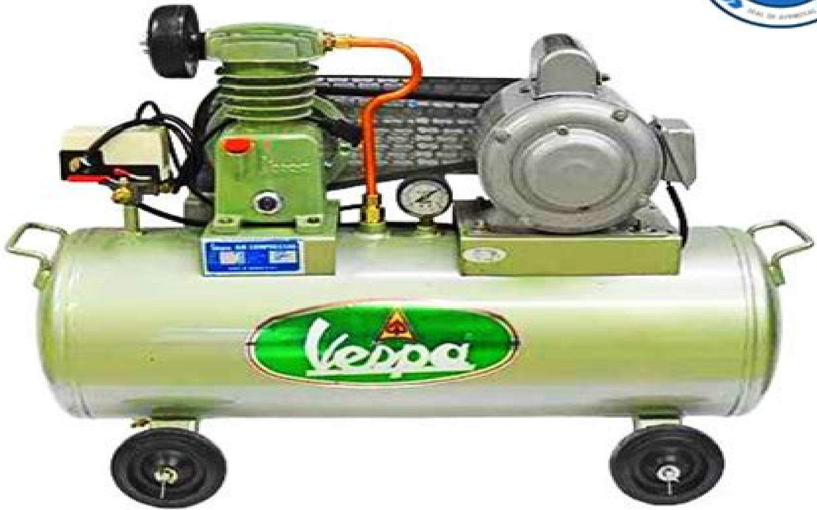
Vespa Air Compressor (1/4 Horsepower)
