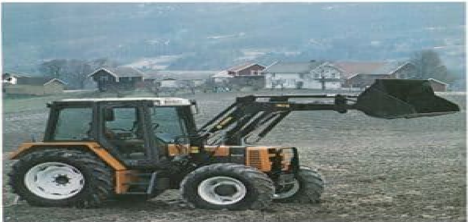
TRIMA 1620, Quick attached loader with parallel linkage and double acting lift rams.
