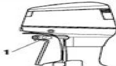
1. Manufactured date label location
