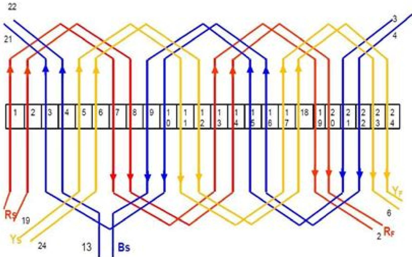
Three phase **AC-Single layer wave winding-24 slot,**
