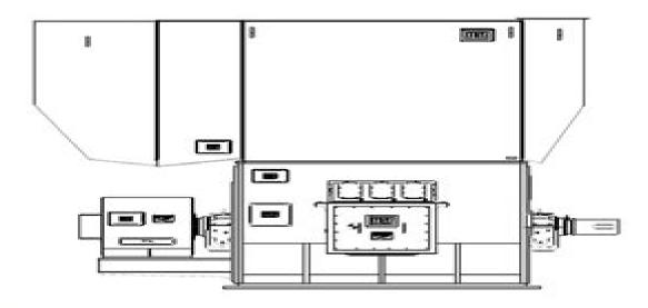
Product: SYNCHRONOUS GENERATOR Model SPI1000 – 15000kVA - 11000V - 50Hz - 4 poles WEG Serial Numbers: 1002688485 - 1002688486 1002284716 - 1002284717
