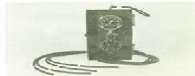
This gauge is needed for carburetor synchronization.
