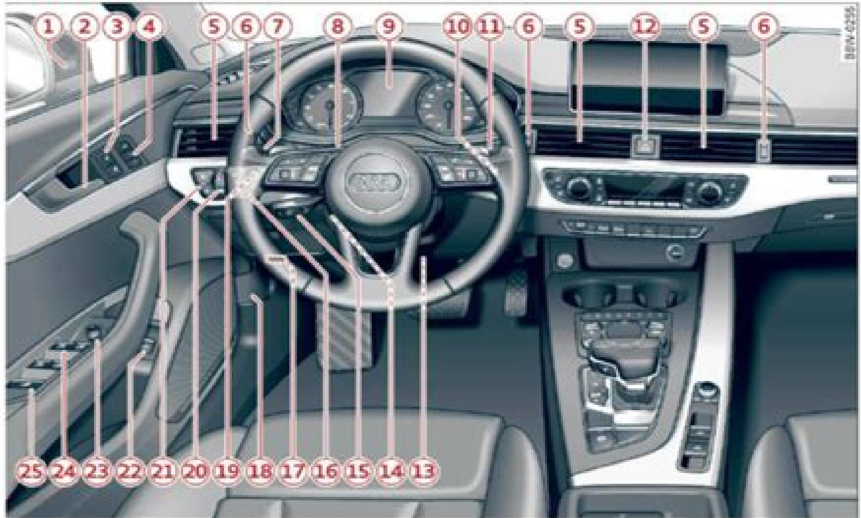
Fig. 1. Cockpit: left section
