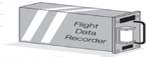
The Black Box, or Flight Data Recorder (FDR)
