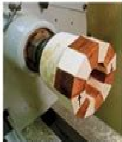
Figure 3-38: Ring mounted to the waste block with hot glue and clamped down
