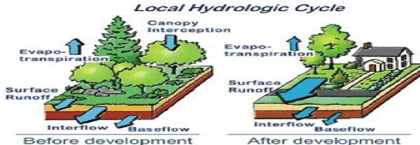
FIGURE 1-7 Schematic of the hydrologic pathways in humid-region watersheds, before and after urban development. The sizes of the arrows suggest relative magnitudes of the different elements of the hydrologic cycle, but conditions can vary greatly between individual catchments and only the increase in surface runoff in the post-development condition is ubiquitous. SOURCE: Adapted from Schueler (1987) and Maryland Department of the Environment; http://www.mde.state.md.us/Programs/WaterPrograms .
